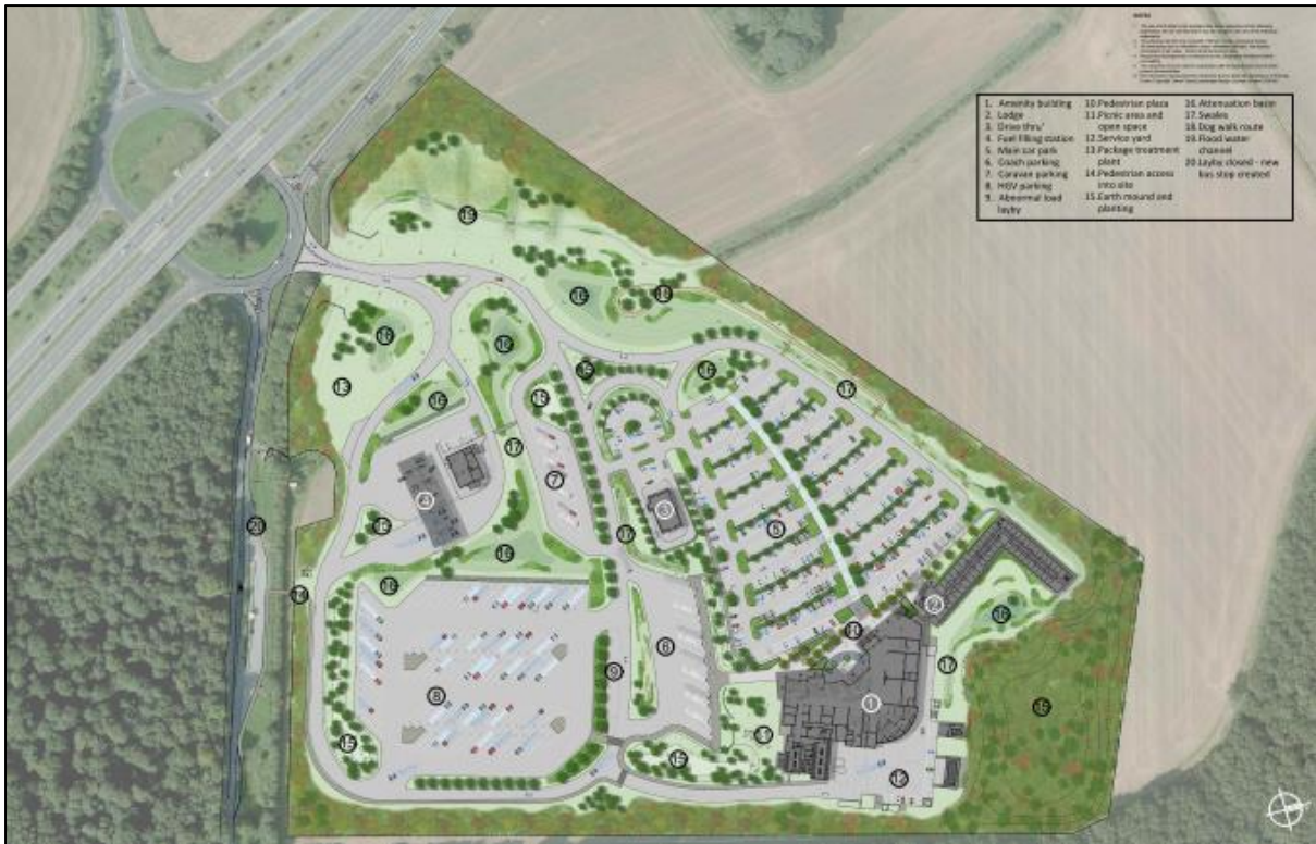
Fig 1: Site layout plan showing amenity building (largest building at bottom right) lodge (I shaped building just to the north of amenity building), drive thru (central), fuel filling station (nearest the roundabout), HGV parking (bottom left) and parking layout.
